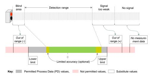
Figure A.6 - Example of a distance measurement Device
