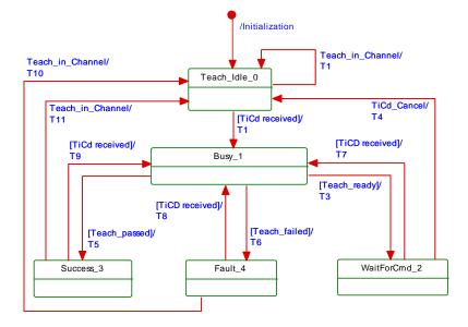
Figure F.12 - State machine of the common teach-in procedure
