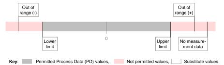
Figure A.4 - Basic Process Data ranges and limits
