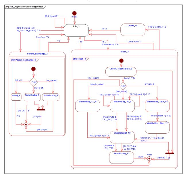
Figure D.2 - State machine of the AdSS proxy FB
