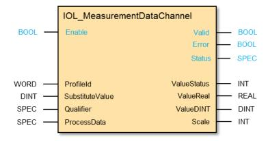
Figure D.3 – Function block for Measurement Data Channel
